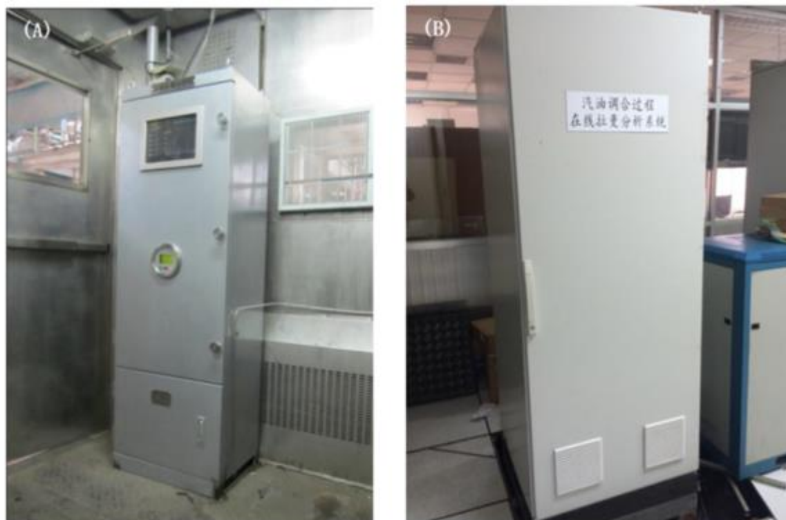
Figure 5. Main cabinet of analysis system: (A). single-channel positive pressure explosion-proof type; (B). Multi-channel non-explosion-proof
