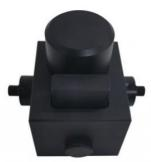
The Cuvette is equipped with quartz collimating lenses, each of which is fitted with a fiber optic connector that connects to an optical fiber to read or illuminate the sample. When used with spectrometers and light sources, it can measure absorbance, fluorescence, scattering, or any combination of the above optical phenomena.
