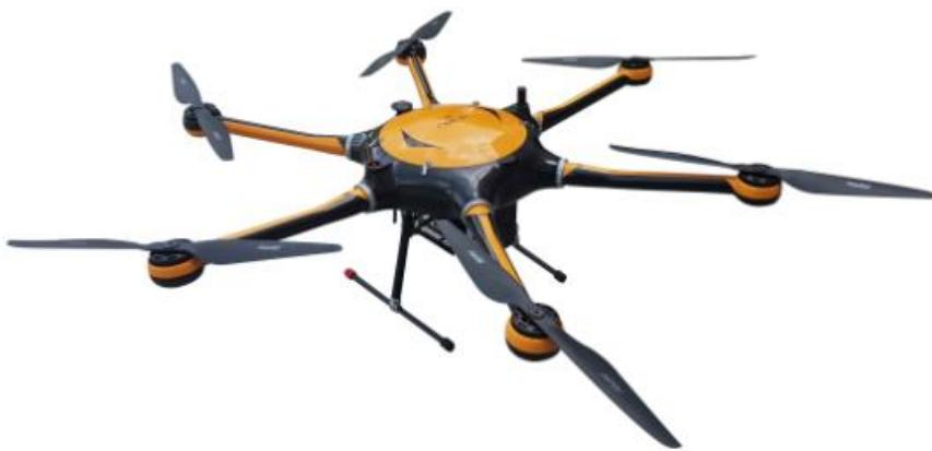
ATH9500 is a series of small, light-weight Airborne miniature hyperspectral imaging system, consisting of a six-rotor high-stability UAV, high-stability gimbal, hyperspectral imager, large-capacity storage system, wireless imaging system, GPS navigation system, ground receiving workstation, ground control system, etc.
