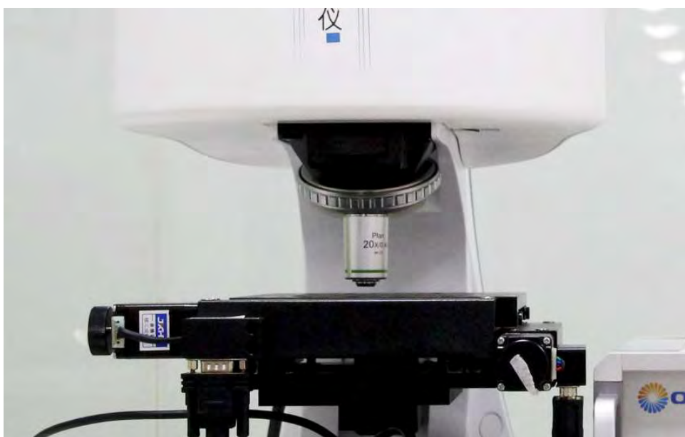
Fig 10 Raman signal high transmission objective, objective focal length up to 8mm
