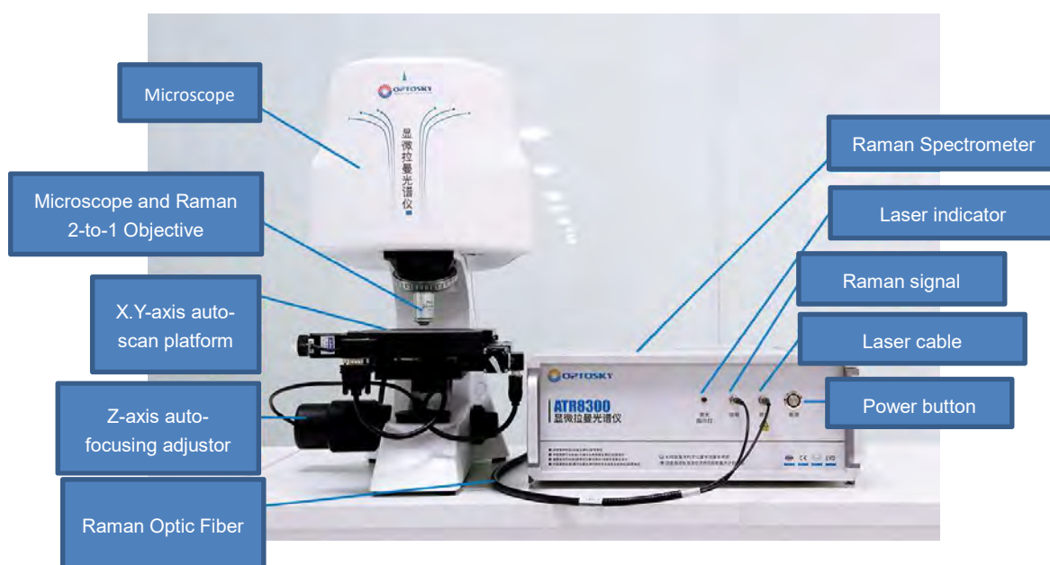
Fig. 1 ATR8300 Structure indication diagram
