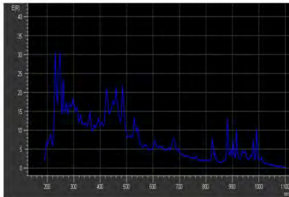
Pic. 1 spectral range (190-1100nm) and power stability
